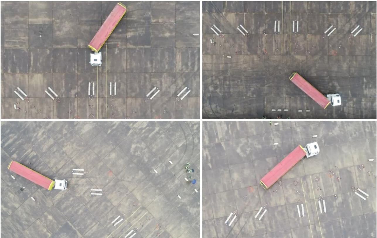
Figure 6 - Manoeuvring a HGV around different charging island designs. Clockwise from top left: Tight turn into 90 degree bay; blind side reverse into 90 degree bay; exiting 45 degree bay; entering 45 degree bay
